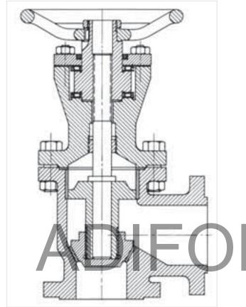
Threaded spindle support mounted between two needle thrust bearings, i.e. AX 45 65 (with matching thrust races) ensures .low frictional characteristics and easy manual operation.
