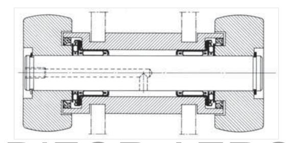
Lubrication is by grease introduced via a nipple on the The common spindle carrying the two rollers turns between two RAX 718 combined bearings (with thrust end of the shaft. plates) which ensures lateral location in both directions.
