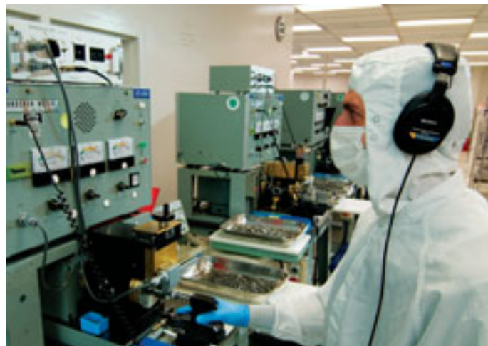
Anderometer, Dynamic Noise and Vibration Tester
